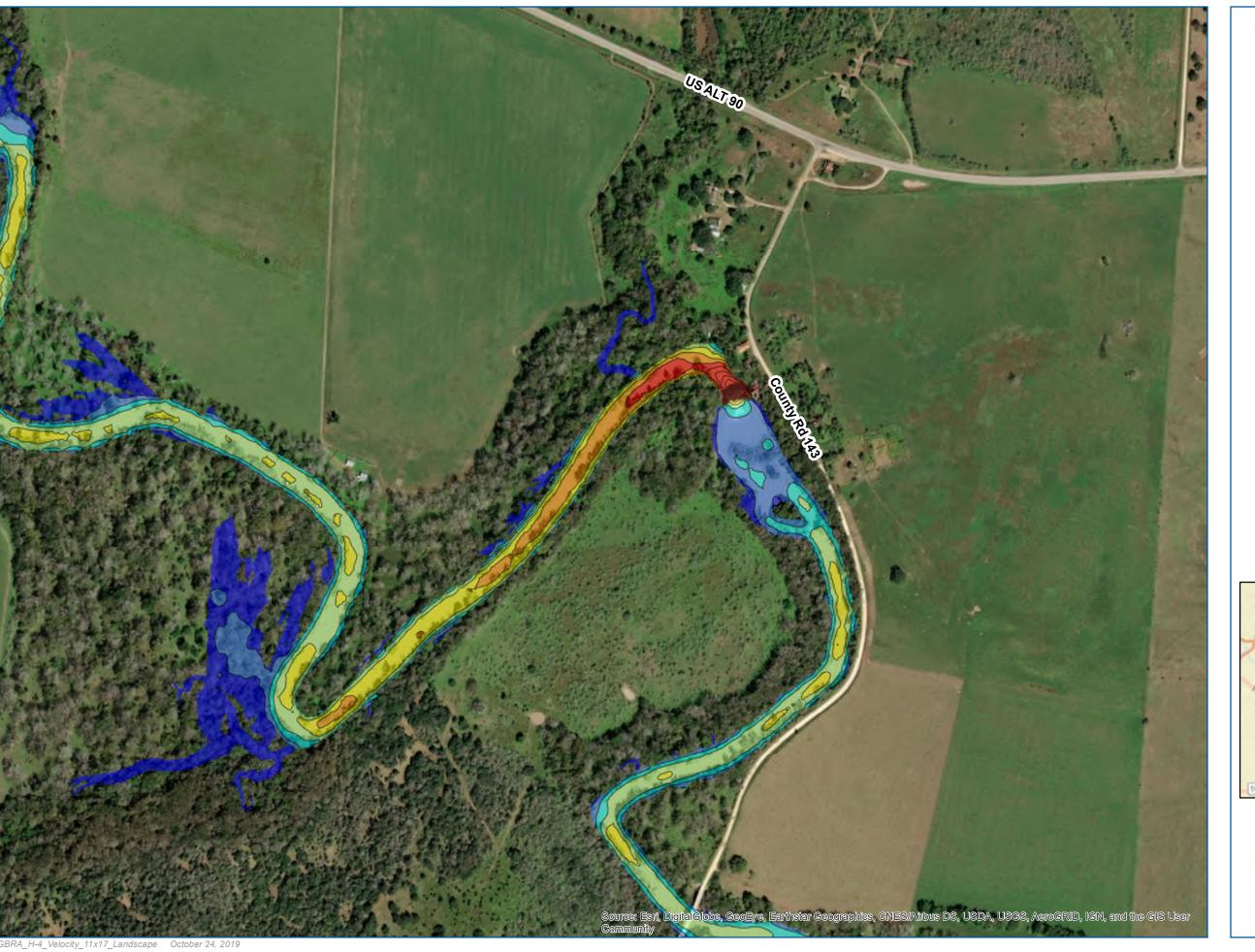
Lake Gonzales Dam (H-4) Dam Failure (1 Gate) Velocity Map
